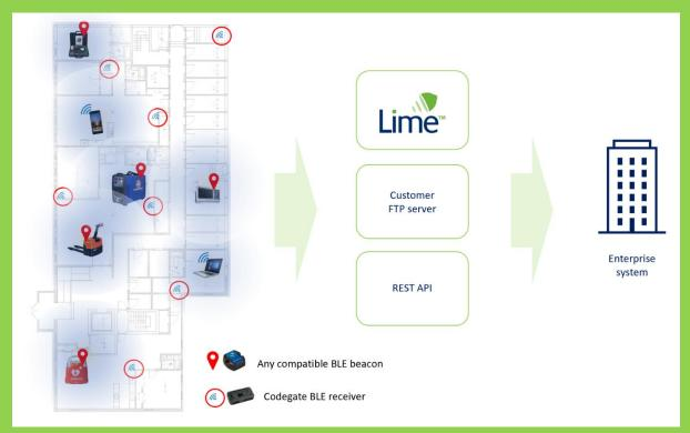
Each eVantage BLE receiver has its own web page, which is user configurable. This allows you to control the signal strength so that stray reads from other floors or areas can be minimised.
